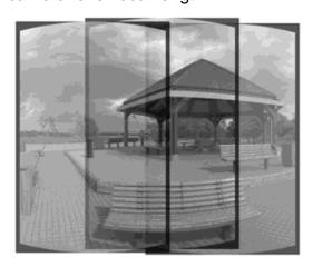
The warped images are overlapped and blended together to create a continuous panorama. Most authoring software uses a search and correlation function, to find the most accurate image alignment automatically. Often manual tweaking of the image parameters by the operator is necessary, but good quality imagery can often be 'stitched' without intervention.
